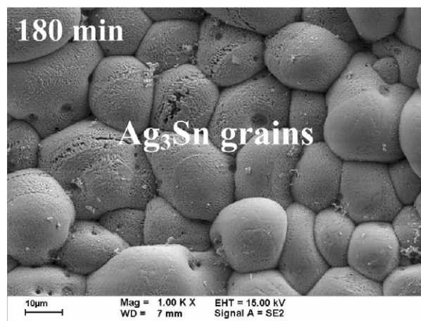
Fig. 2. Top-view SEM micrographs of the Ag 3 Sn grains formed at the 90Pb10Sn/Ag interfaces reacted at 350 °C for (a) 5 min and (b) 180 min.
